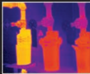
Failed Steam Traps
